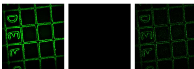
Figure 1: Third harmonics of a calibration grid (Ibidi) with 50 micrometer squares. a) 4.7 mW, full spectrum short pulses (<50 fs). b) 6 mW with laser spectrum limited to 10 nm bandwidth (~160 fs). c) Scaled up contrast for the 6 mW laser spectrum limited to 10 nm bandwidth (~160 fs).
