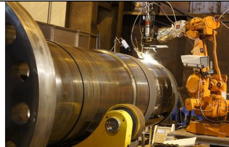
Laser cladding. Metal structure with the help of laser technology allows for increased product performance and meet the demands of extreme surface and function of the characteristics of friction, corrosion, wear, etc.
