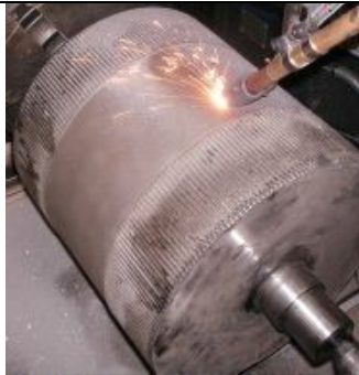
Roller grooves rebuilt by Laser Cladding. The welding material is wear resistant tool steel mixed with hard, wear-resistant ceramic and particles.
