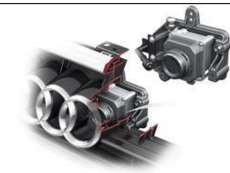
The Night Vision sensor is typically mounted in the grille as seen in the image to the left.
