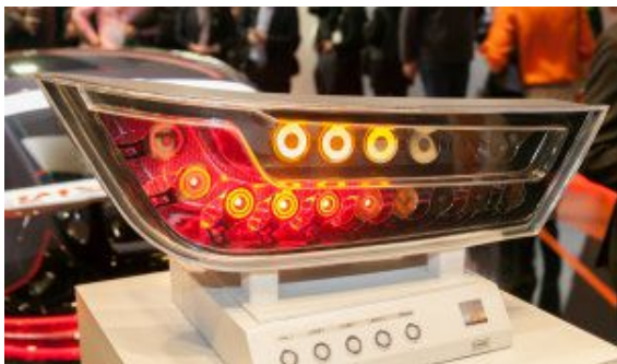
LED/OLED rear light automotive demonstrator showcasing four lighting functions – brake light, turn indicator, reversing light and rear light.
