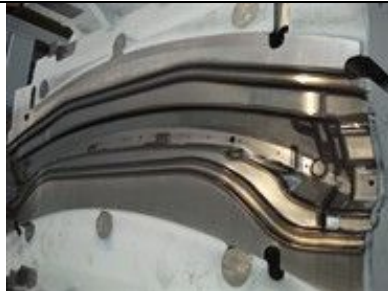
Details that need to be partially cured. Pictured tool part where wear exposed radii are laser hardened.
