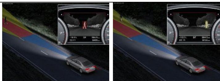
The Night Vision system will warn the driver if a pedestrian is present in the danger zone (marked in red) in front of the vehicle. The width and length of the danger-zone are dynamic and depend on speed of the vehicle. (Image credit: Audi).
