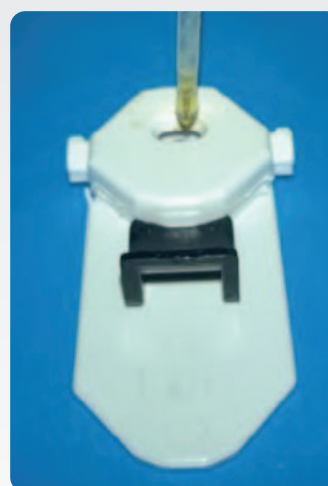
Figure 21: Disposable fiber sensor receiving a sample drop. Credit: Diafir.
