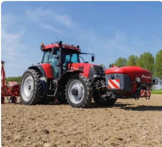
Figure 11: The iXtra LiFe is responding to photonics data by liquid fertilizing. Credit: Kverneland.
