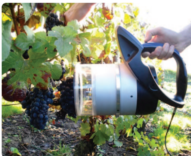
Figure 9: Sensor measuring anthocyanin on grape bunches. Credit: Force-A
