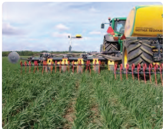
Figure 12: The camera-aided Cameleon machine means precision. Credit: Gothia Redskap
