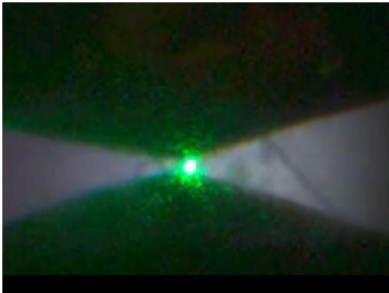
Fig 1. Water droplet trapped between two neodymium magnetic tips illuminated by a 532 nm low-power laser.
