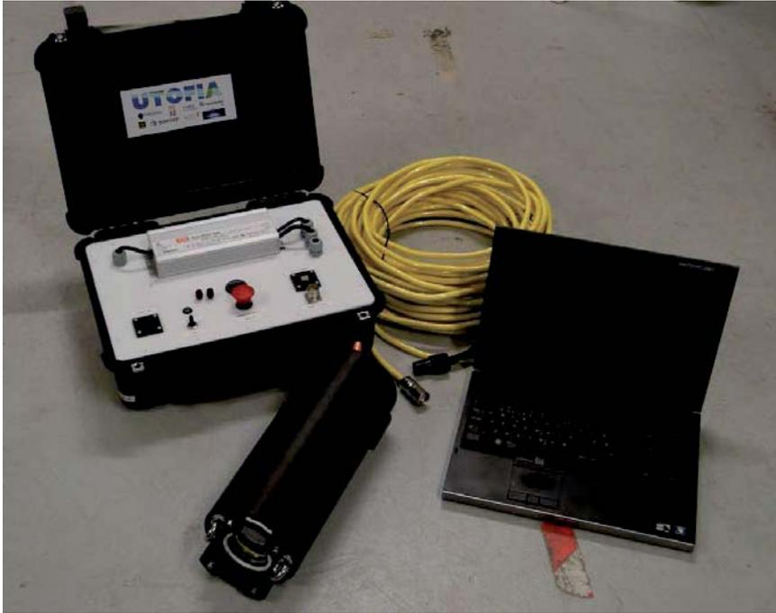
**UTOFIA System Two; subsea camera unit (lower left), topside power, umbilical cable and PC.**
